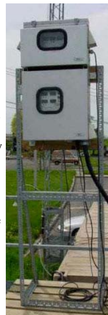
This Tekran sampling unit in Elizabeth measures elemental, reactive gaseous, and particle-bound mercury. Units are also installed in Camden, New Brunswick, and Chester.
